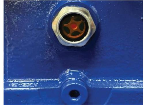
**Figure 4.3.** Oil Drain Plug
