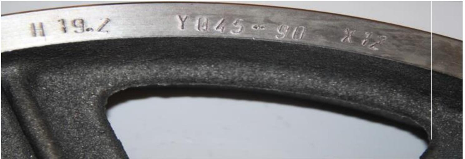
**Figure 16.2.** Traction Pulley Coding Example
