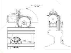
Figure 11.1 Rope wrapping angle for Machines
