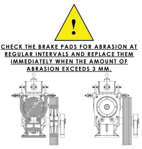
Figure 7.4. Brake Jaw and Pad
