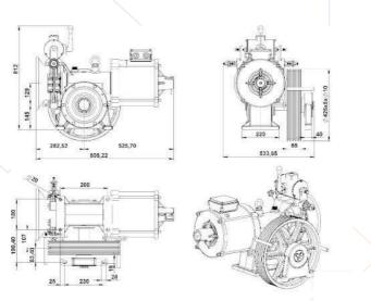
Figure 19.10. Mugen Machine Installation View
