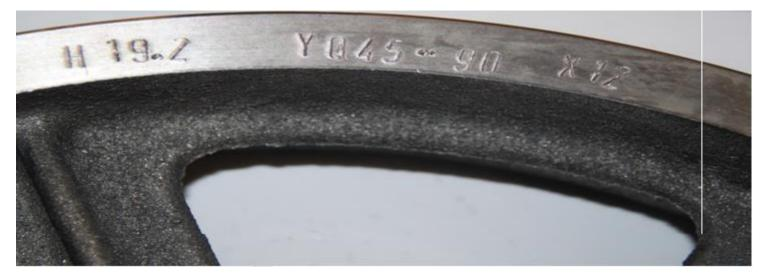
Figure 16.2. Traction Pulley Coding Example
