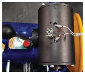
Figure 7.2 198 v DC Brake connection
