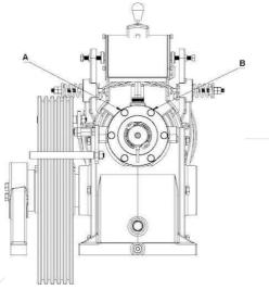
Figure 14.1.Axial Bearing Adjustment
