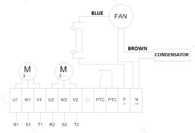
Figure 5.4. Double Speed Connection with Fan
