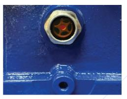
Figure 4.3. Oil Drain Plug
