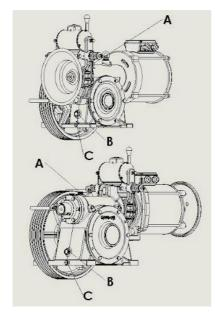
A: Oil Filling Reservoir B: Oil Indicator C: Oil Drain Plug
