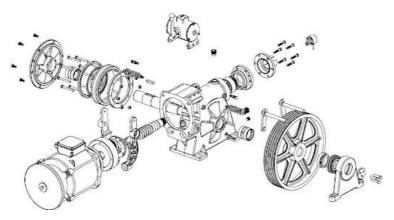
Figure 19.3. Display of Volpi Machine Components
