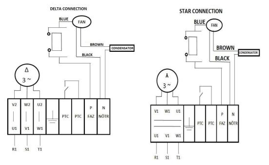
Figure 5.2. Single Speed Connection with Fan
